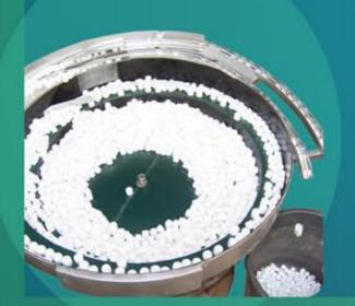
We manufacture bowl feeder from a small 200mm. diameter bowl to 1000mm. diameter bowl in M.S. or S.S. Each bowl is designed and manufactured according to the need of customer to give proper orientation and trouble free service.
