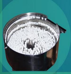
Vibration has been a very fascinating subject for man since ancient times. With the advent of new technologies, man has mastered the art of creating and controlling vibrations. In our design of the vibration bowl feeder, the vibrations are created in spiral fashion so that the components placed on the bowl which is fixed to the vibrating unit start moving round and round. The bowl being custom built for the particular component, has a peculiar geometry.
